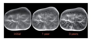
Fig. 2 REM documentation on glaze wear over three years (source: Courtesy of TRAC Research Clinical Studies Section, CR Foundation, Provo, Utah USA)
